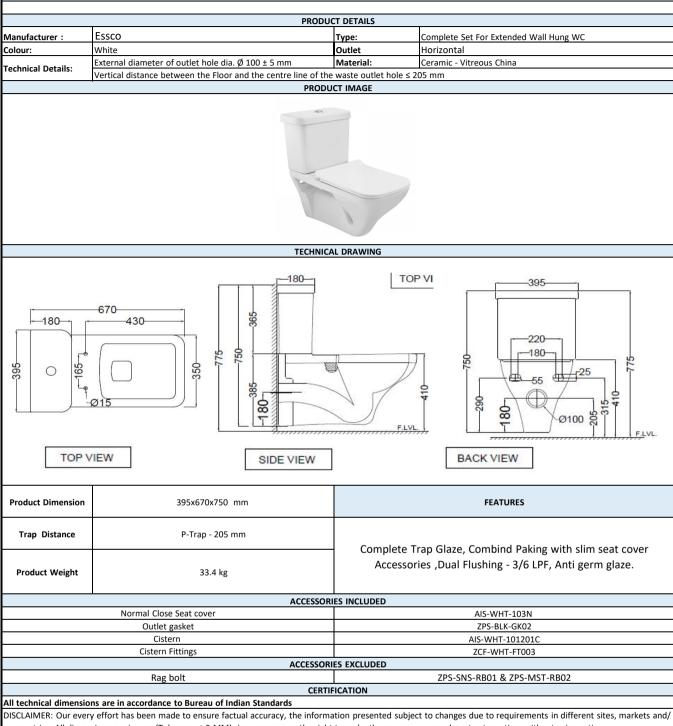
or countries. All dimensions are in mm (Tolerance ± 5 MM). Jaquar reserves the right to make the necessary amendments at any time without prior notice.
